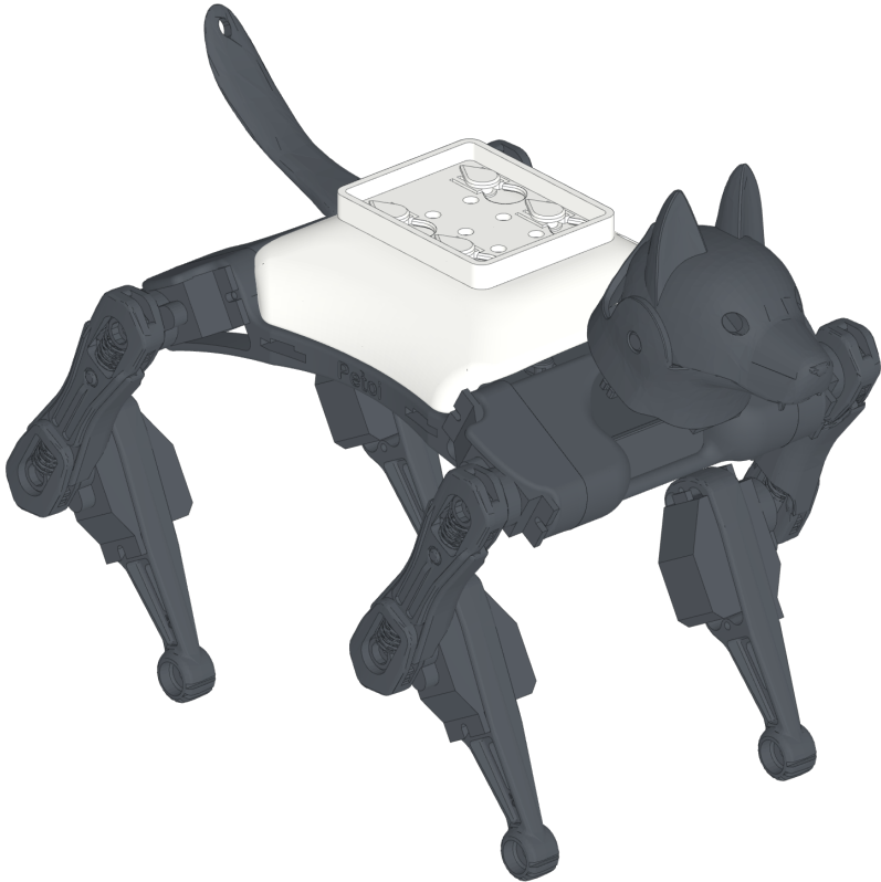
The platform (white) on the robot, with the starter plate on the pegs.
